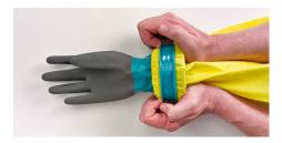
Step 7 - Using both hands push the AlphaTec\* ribbed green collar further up the sleeve until tightly locked in position. Ensure outer ring is tightened as far as possible to provide a secure fit.
