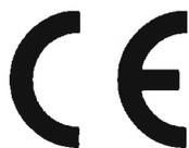
To the CE marking of PPE of category III will be added the identification number of the notified body carrying out the control measures.
